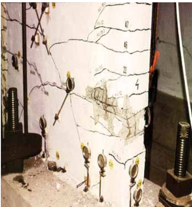
Figure 10. Precast concrete shear wall after failure.
