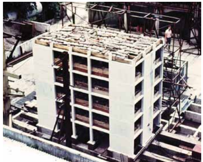
Figure 12. Five-story precast concrete structure (model scale 1:4) during shake table tests.
